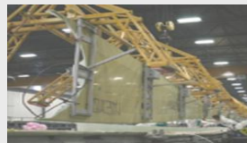
Assembling spar web on the shell mould
